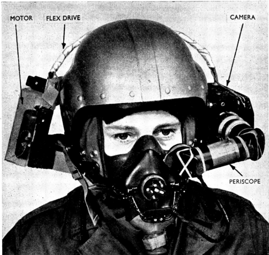
FIG. 6. Apparatus for measurement of rotational eye movements.
